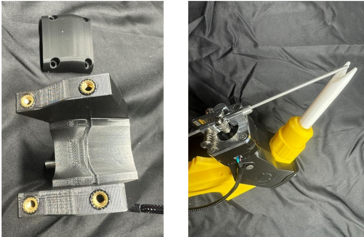
Figure 2. Bottom and top mount assembly. Note the alignment ridge (left) and free rotation of the nozzle attachment nut (right).
