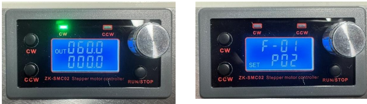
Figure 3. Control box during normal operation — CW indicator illuminated, Setting 60 (14 in/min), F-01 P02 drive mode.
