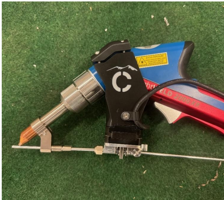
Figure 1. LASER_TUG rod feeder mounted to IPG LightWeld handheld laser welder
